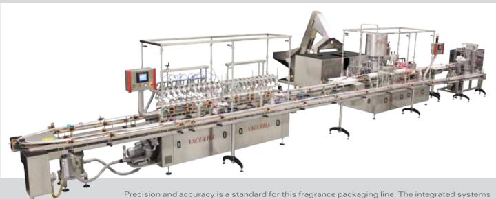
Precision and accuracy is a standard for this fragrance packaging line. The integrated systems are configured to fill, crimp pump units, place spraying actuators, over cap, and label perfume container. To add flexibility and reduce change-over time, the line is designed to also handle pucks. Redundant inspecting systems are also integrated to ensure process compliance.
